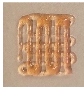
Figure 10.10.19: A 2-layer lattice printed through a 25G (I.D. = 0.26 mm) needle. Light crosslinking was performed after deposition of each layer, to strengthen the structure.
