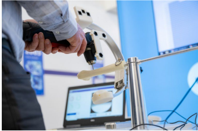
Figure 10.9.1: DEHST prototype for training of free hand distal interlocking, exhibited at AO Davos Courses.
