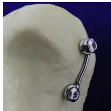
Figure 11.3.4: Implant prototype, capable of applying constant force to the physis, mounted on a plastic bone.
