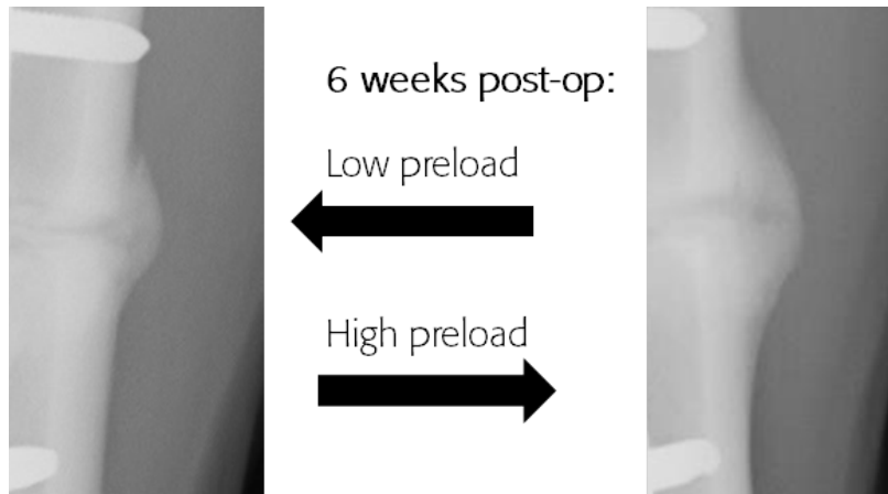
Figure 9.3.1: Anteroposterior (AP) Radiographs at 6 weeks post-op of two animals. Left: low preload (12.5 kg) applied to the spring of the fixator; right: pre-load to the spring of the fixator increased to 25 kg. A more pronounced callus formation becomes obvious for the high-preload animal.
