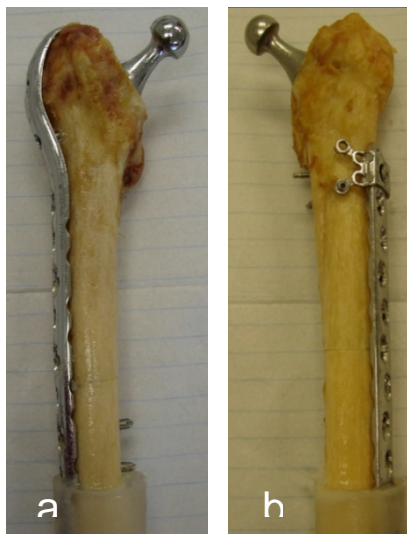
Figure 9.5.3: Specimens prepared for biomechanical testing with a hook plate (left) and LCP with locking attachment plate (right).
